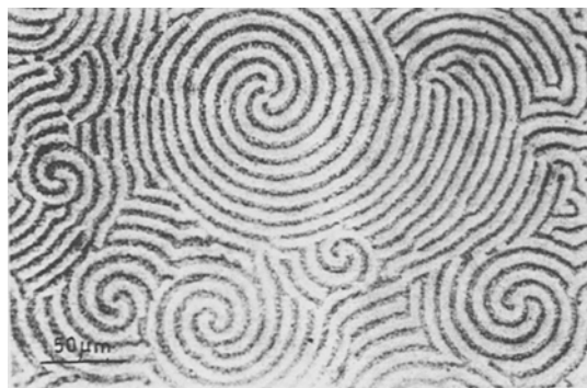
Fig. 3. Spiral waves with different topological charge with connected and disconnected arms, plated at 1.5 \text{ A dm}^{-2} with 6 \text{ g l}^{-1} antimony in the electrolyte.
